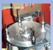
Optional: Measure a lot of powder samples inline by using the sample change.
