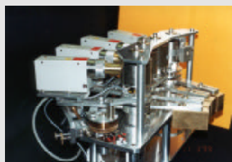
Fig.1: The compact unit of the multiple-detector system. The middle stage carries the crystal analysers and detectors. The top plate holds the analyser shielding houses.
