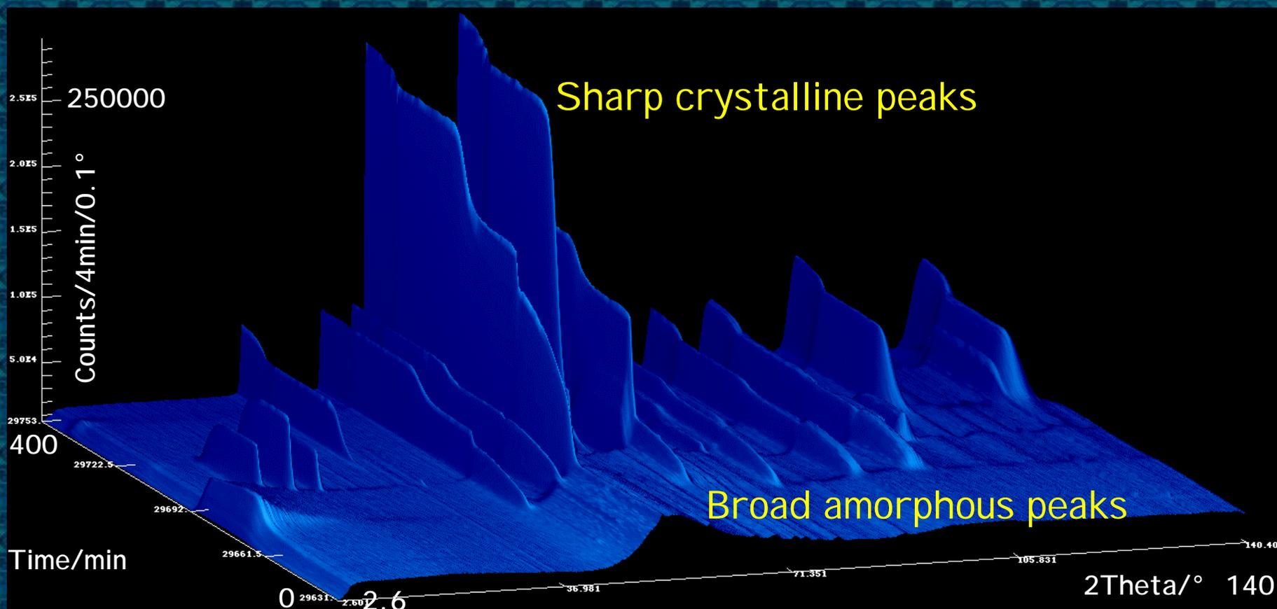
Complete diffraction pattern in minutes or seconds, scanning through temperature
