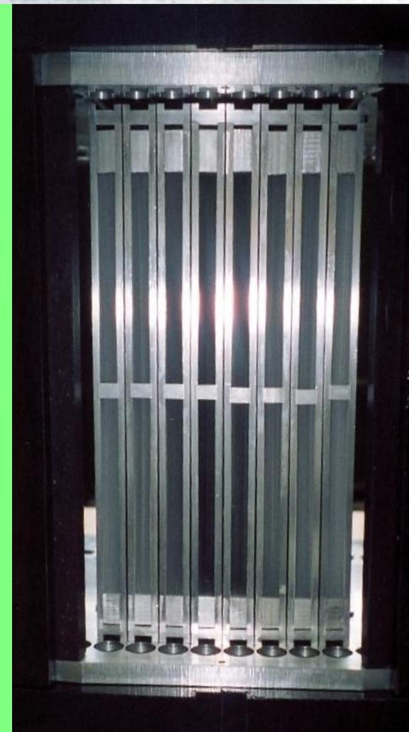
128 x 300 mm high resistive wire detectors, high resolution collimators
