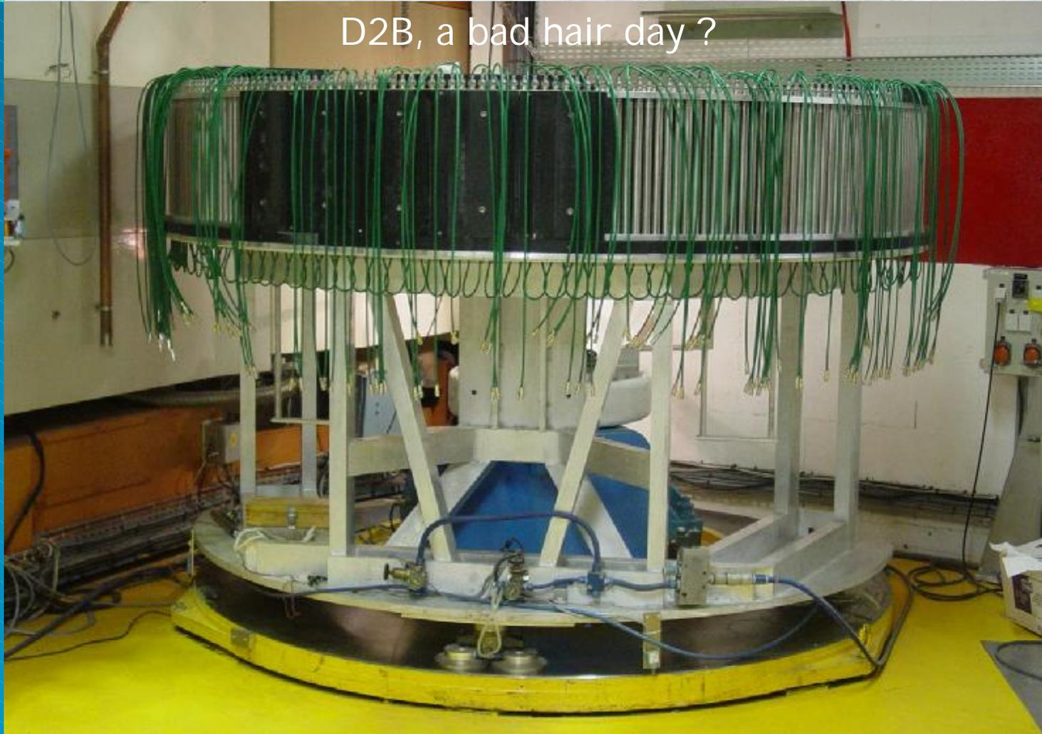
128 x 300 mm high resistive wire detectors, high resolution collimators
