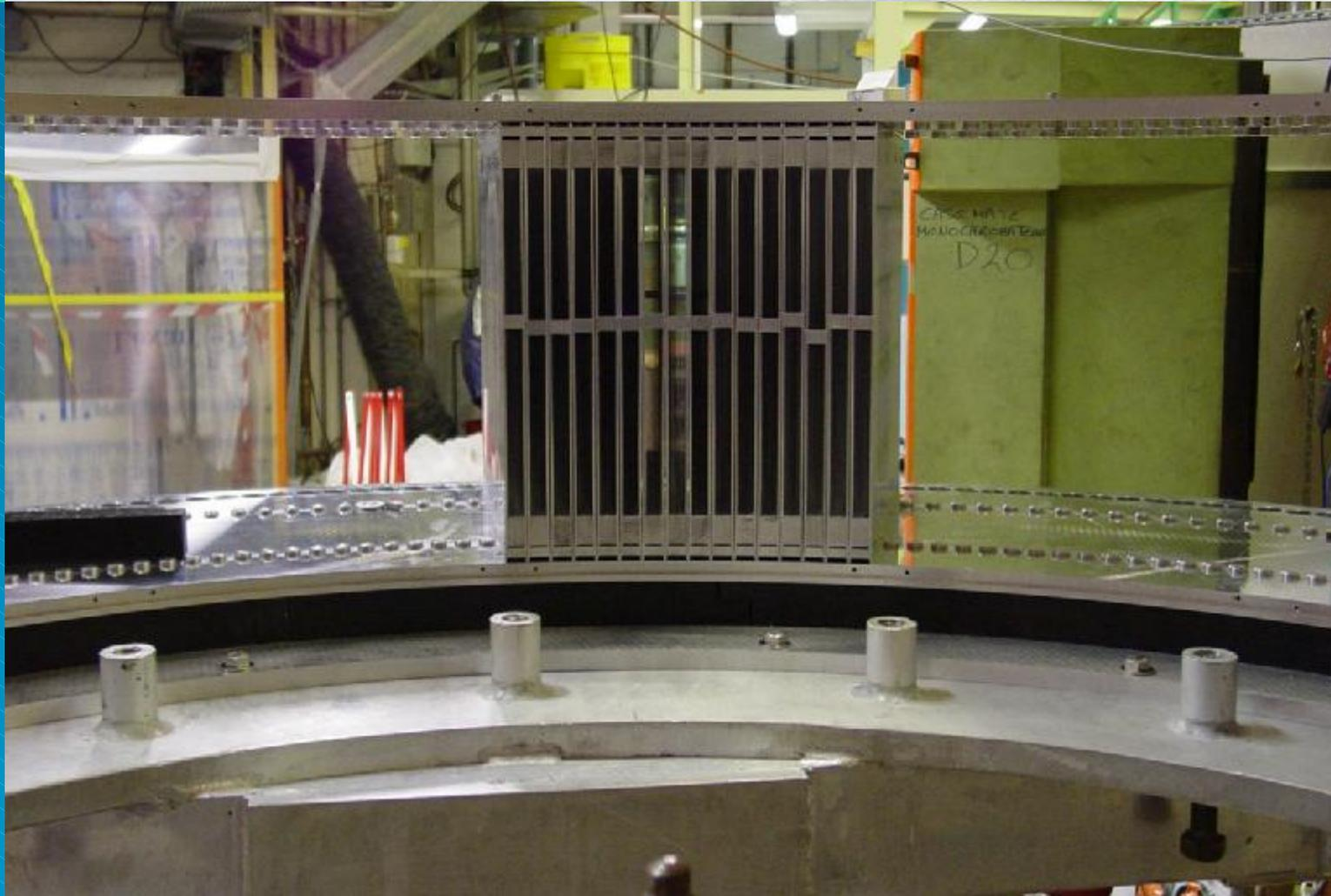
128 x 300 mm high resistive wire detectors, high resolution collimators
