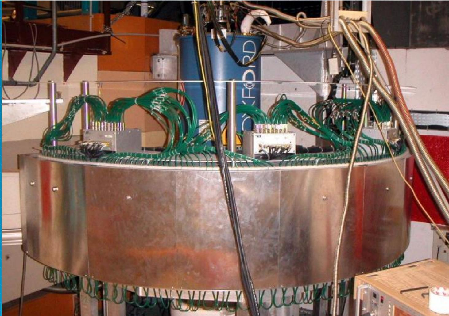
Completed 300 mm high 2D-detector, with 6 Tesla cryomagnet
