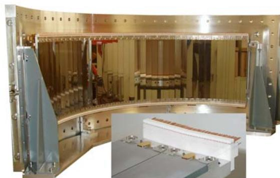
Fig. 9 A very large 2D PSD for D19, showing arrays of linear sensitive wires in front of electrodes deposited on glass (inset).
