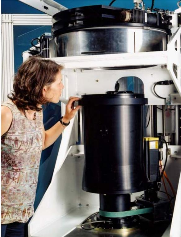
Fig. 2 VIVALDI combines high flux on the sample using a continuous white beam with a very large image plate detector.
