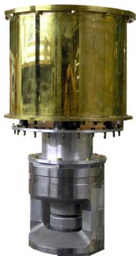
Fig. 14 The new 100 kbar pressure cell with its He cryostat.
