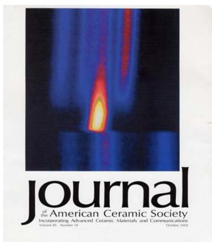
Fig. 7 The explosive SHS reaction in  $\text{Ti}_3\text{SiC}_2$  on D20. The intermediate phase (bright spot) lasts only ~1 second.
