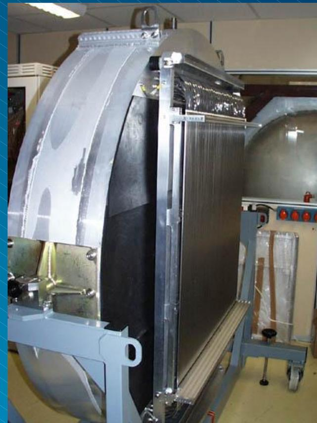
Array of 8mm x 1000mm linear wire detectors, D22
