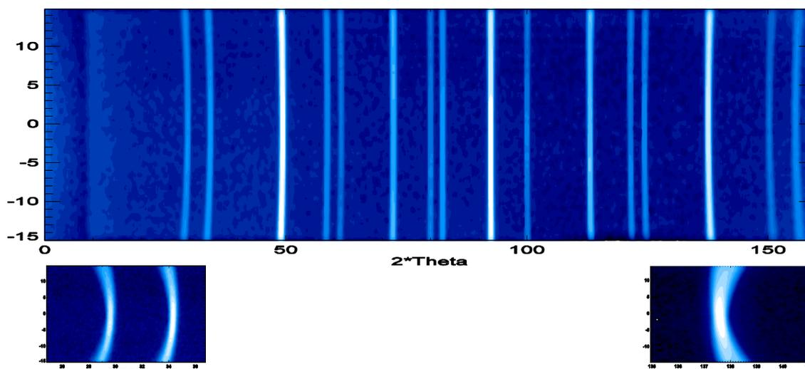
**Fig. 7.** High resolution powder data from a large 2D detector, showing the curvature of the diffraction cones (Suard et al 2003).
