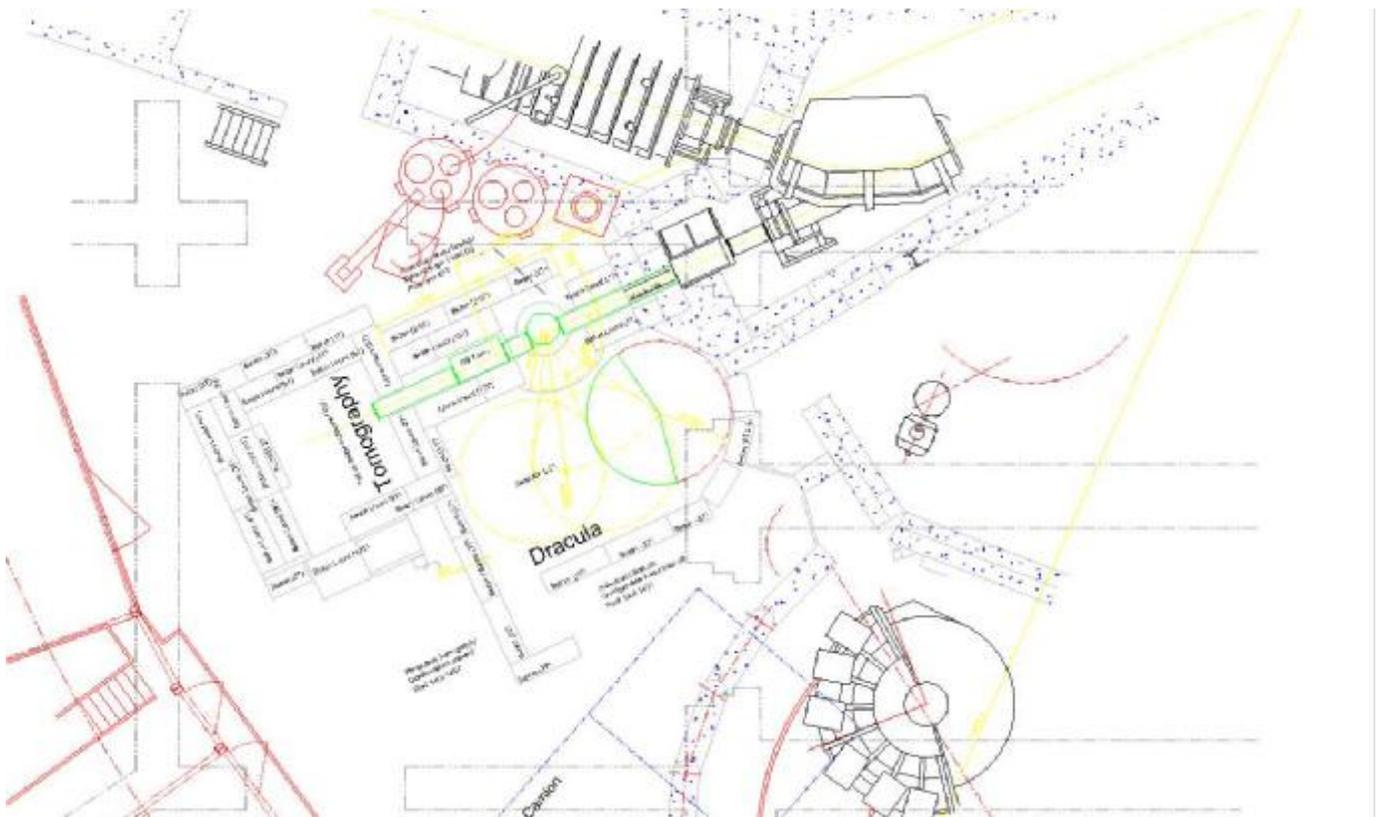
**Fig. 1b** Option B: Dracula would displace the tomography station on the 200mm diameter high flux H9 Lohengrin beam tube. The H9 beam tube is perhaps the most intense thermal neutron beam anywhere, and if we are to compete with the American pulsed source this position must be used to maximum advantage.
