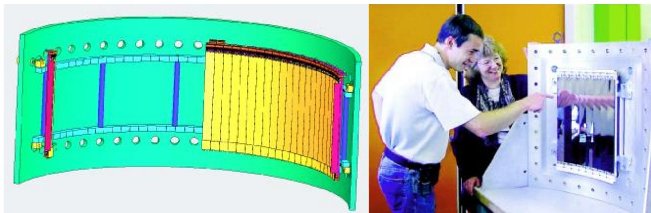
**Fig. 6.** The new 30°x120° 2D-PSD for D19. Large detectors match the solid angle of the best pulsed-neutron diffractometers, while benefiting from the very high flux available on the sample at a reactor source. (Guerard et al. 2002).
