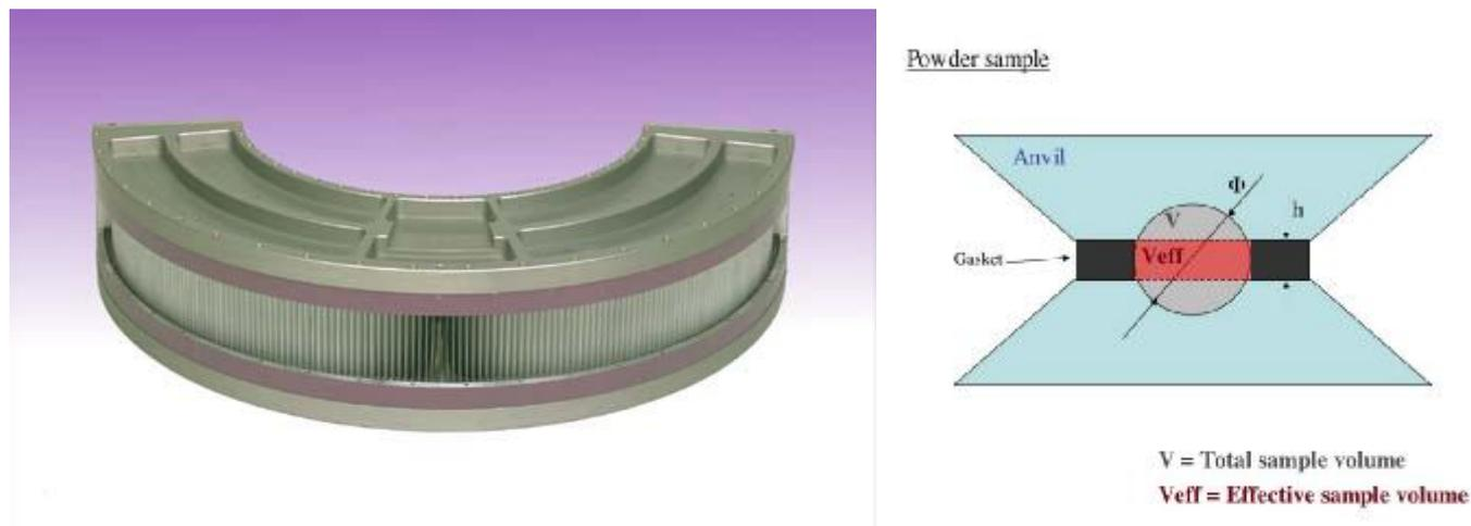
Fig. 4 Radial collimator of the type to be used for Dracula 2(b) High pressure Paris-Edinburgh cell being constructed for ILL.
