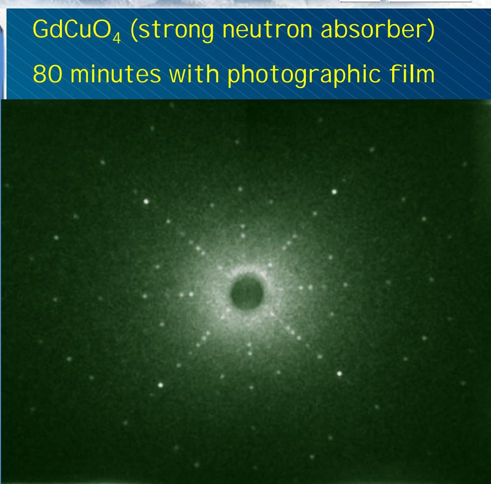
90 seconds with neutron CCD camera
