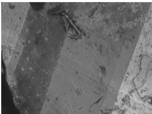
FIG. 2. Image of twinned natural proustite NPr1 under crossed polars.
