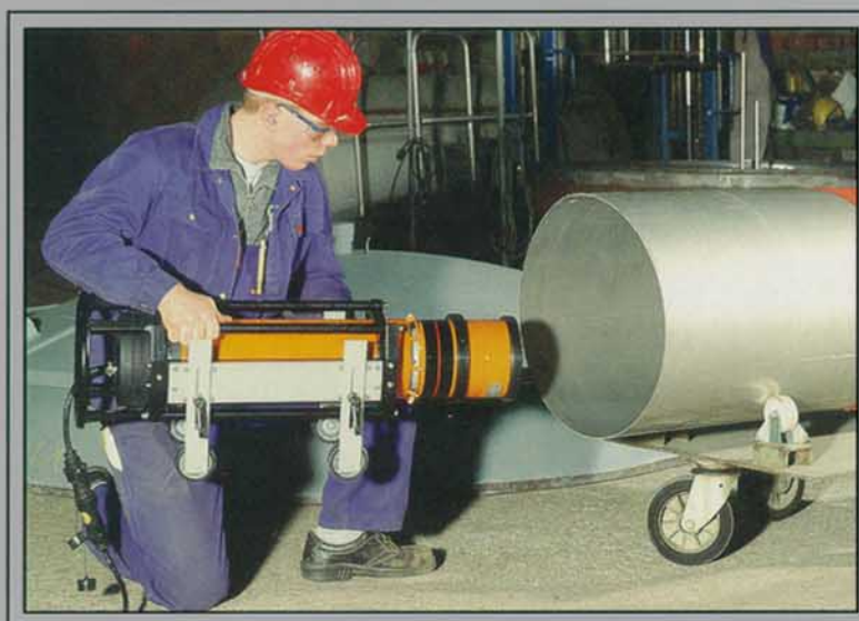
X-ray equipment of the ERESO MF line being set up for various inspection tasks.
