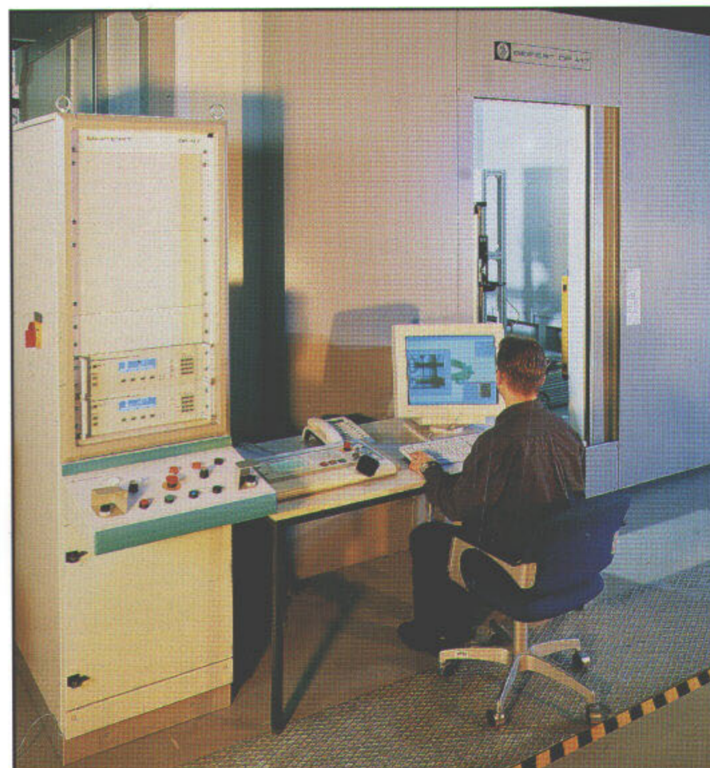
DP 417: Radiation protection cabinet for up to 450 kV X-ray voltage
