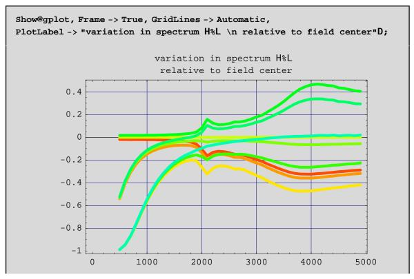
The spectrum viriation is asymmetric, as expected. It is easy to recognize the 3 cases; at low energy, the three "right" filed positions correspond to the lowest 3 curves (thicker Be suppresses lower energies).
