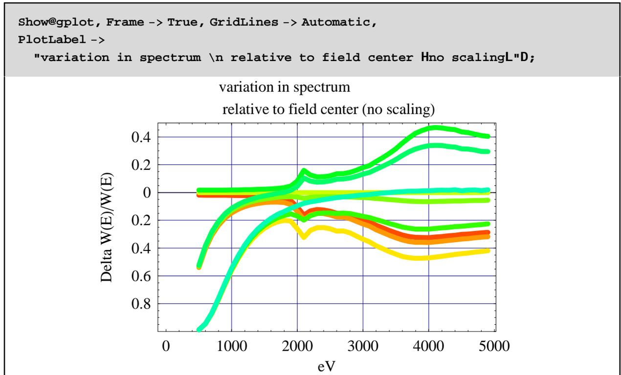
The spectrum variation is asymmetric, as expected. It is easy to recognize the 3 cases; at low energy, the three "right" filed positions correspond to the lowest 3 curves (thicker Be suppresses lower energies).
