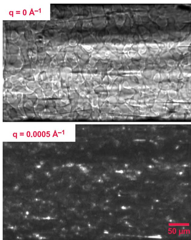
**Figure 2:** USAXS images from a slow-cooled tissue engineered scaffold acquired with  $q = 0 \text{ \AA}^{-1}$  (upper panel) and  $q = 5 \times 10^{-4} \text{ \AA}^{-1}$  (lower panel).
