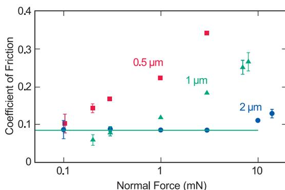
Figure 1: Effect of tip sizes on friction.
