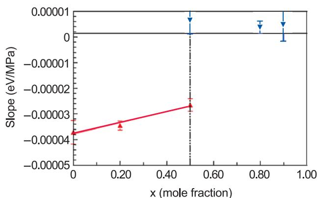
**Figure 4:** Slopes (i.e., peak position/stress) of PL lines as a function of composition. In the left side of the figure, PL results from direct transition; in the right side, PL results from indirect transition.
