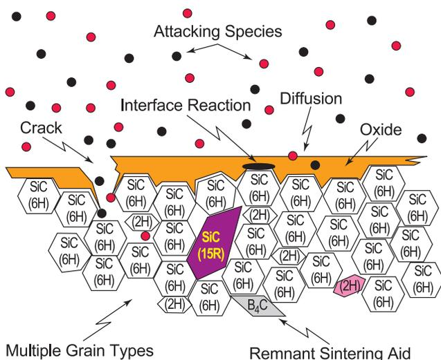
**Figure 1:** Data evaluation must account for the complexity of polycrystalline materials and the resulting dependence of material properties on chemical composition, physical microstructure, and environmental conditions.
