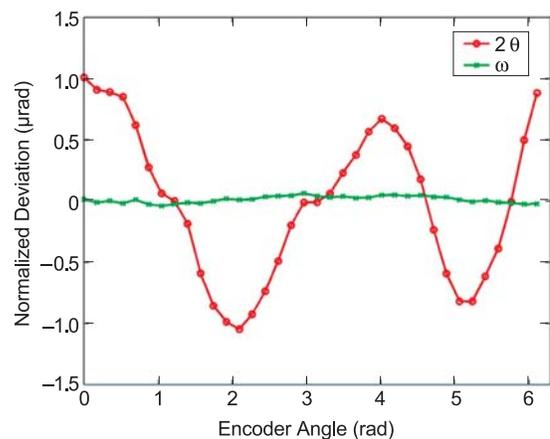
**Figure 2:** Encoder error corrections from circle closure.
