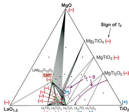
**Figure 1:** Subsidiary phase relations in the  $\text{La}_2\text{O}_3\text{-MgO-TiO}_2$  system (air;  $\approx 1450^\circ\text{C}$ ), sign of the temperature coefficient of resonant frequency ( $\tau_f$ ; in parentheses), and approximate locations of two regions of temperature-stable ( $\tau_f = 0$ ) equilibrium mixtures (dotted lines).
