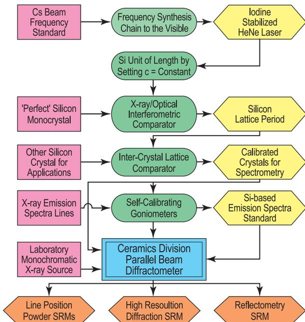
**Figure 1:** Measurement chain of NIST certified diffraction SRMs.
