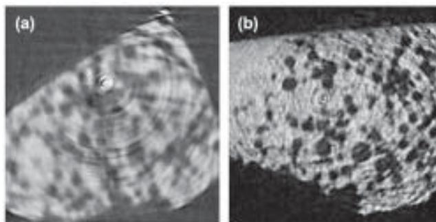
**Figure 1:** XMT single-slice images through a SOFC anode layer at (a) 17 keV and (b) 27 keV x-ray energy. The 27 keV image exhibits a strong contrast between the Ni and yttria-stabilized zirconia components.
