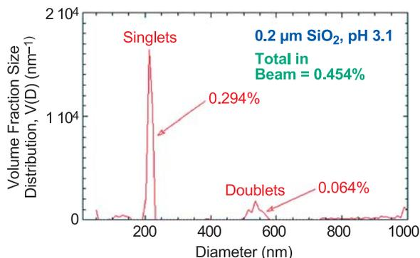
**Figure 1:** Volume fraction PSD for SiO<sub>2</sub> at the isoelectric point.
