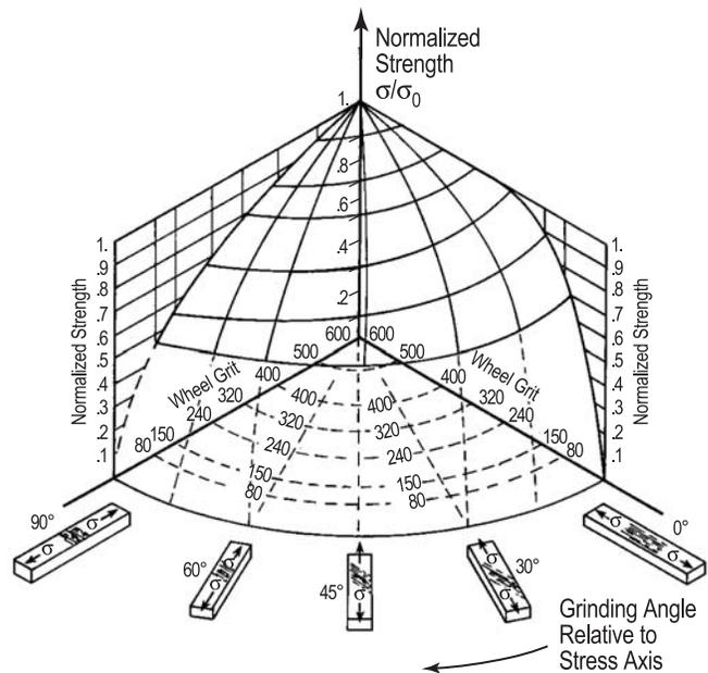
Figure 1: Grinding damage map for silicon nitride.
