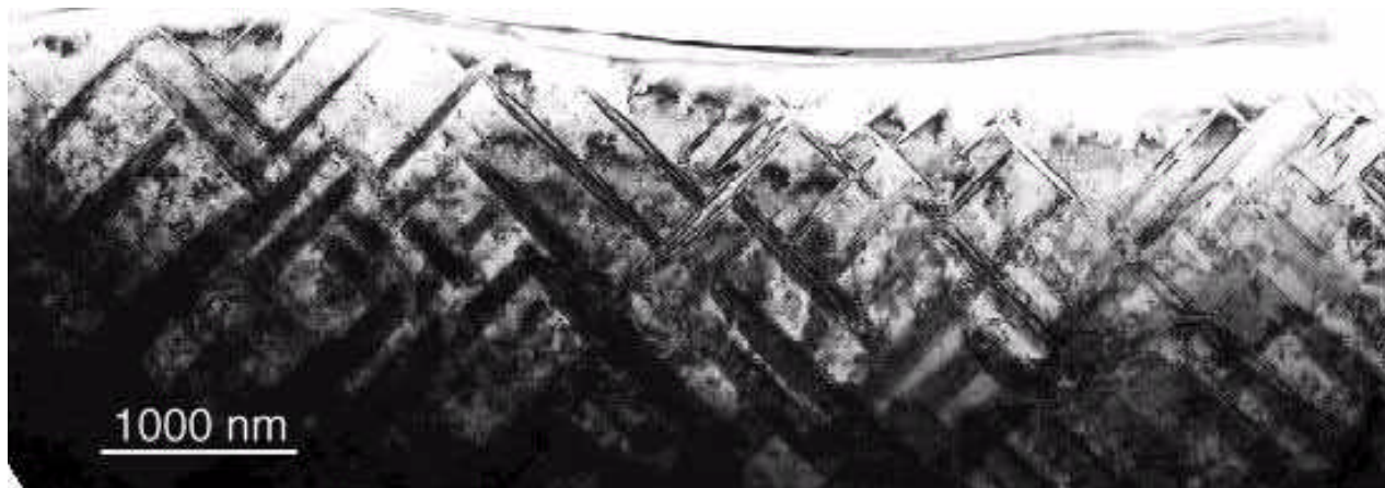
Cellular 3-domain Structure (500 nm PZT 20/80 on SrTiO 3 )
