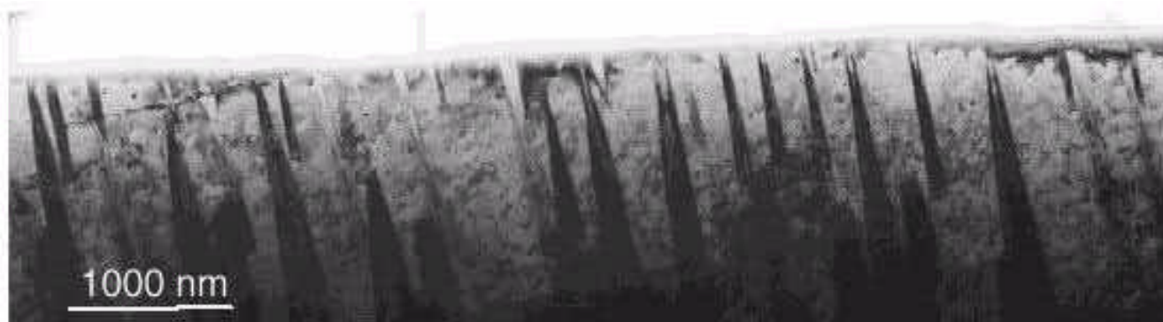
c/a/c/a 2-domain Structure (200 nm PZT 20/80 on SrTiO 3 )
