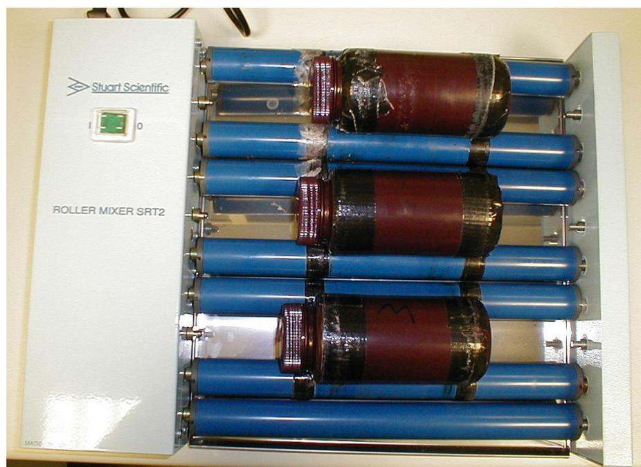
**Figure 2.2.** Picture of the batch reactor set-up for all dissolution experiments, where the rollers rotated at a fixed speed of 33 rpm, and rose and fell 16 mm.
